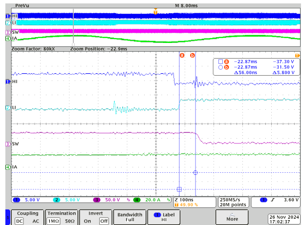
Figure 4-15. Phase U Falling SW, Phase Current 36V, 20A
