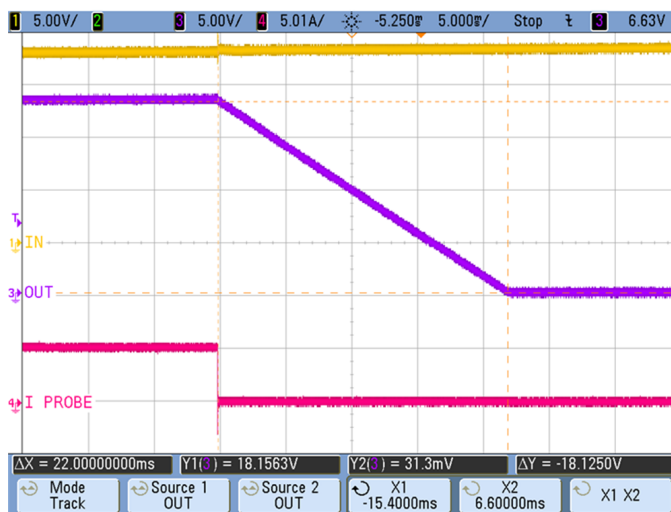
Figure 3-1. Over-Voltage Protection Cut-Off Mode
