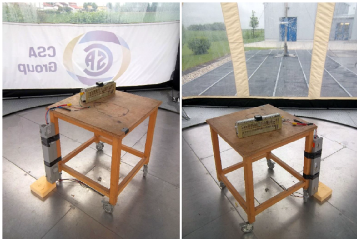
Figure 29. Radiated Emission 10-m Test Setup
