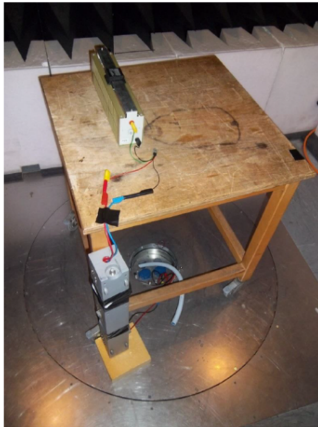
Figure 26. Radiated Emission 3-m Prescan Test Setup
