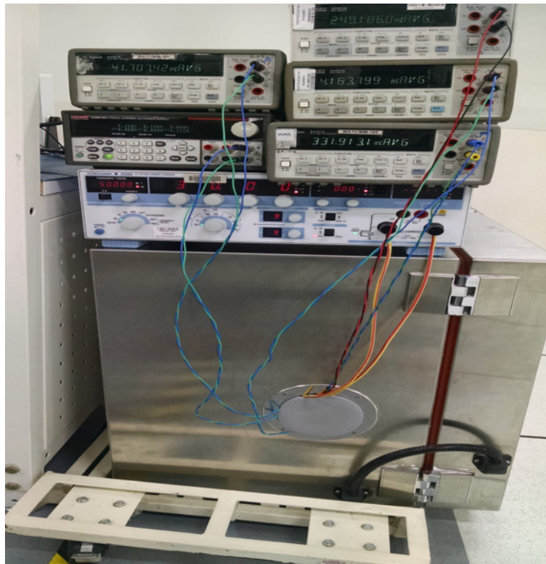
Figure 16. Test Setup for Testing Over Temperature Range
