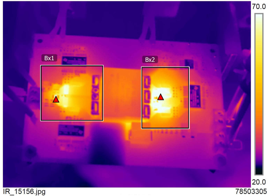
Figure 2-4. Thermal Images, 36-V Input, Top of Board
