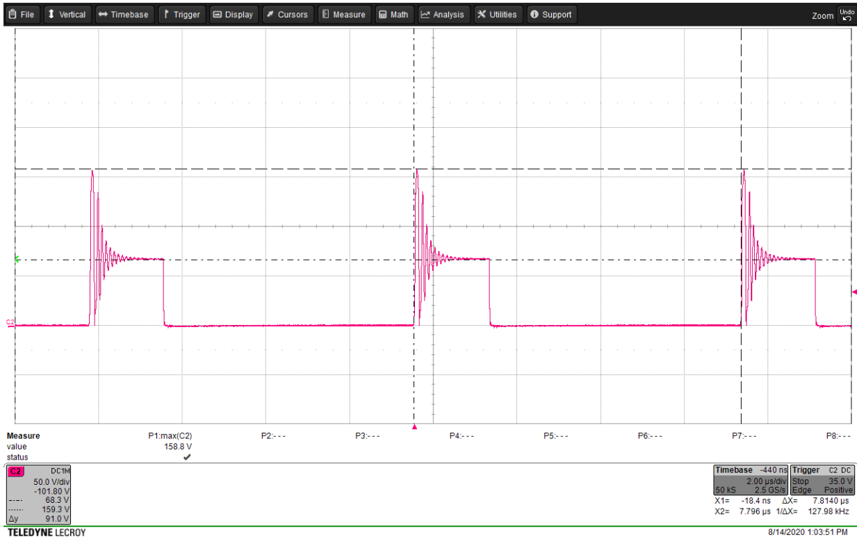
Figure 3-2. 19 VDCin; 24 V OUT at 420 mA
