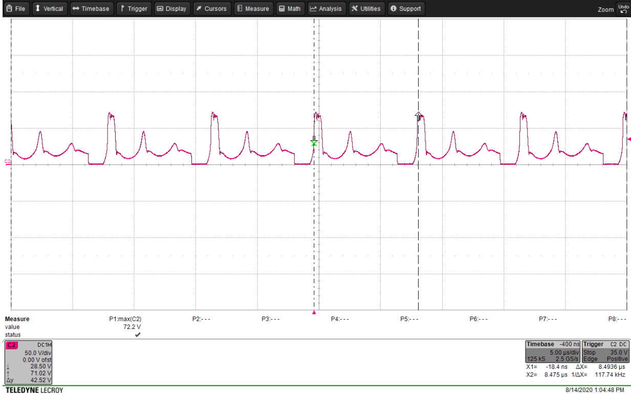
Figure 3-1. 19 VDCin; 24 V OUT at 0 mA
