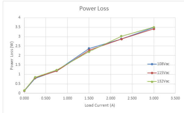
Figure 2-2. 20-V Output Power Loss
