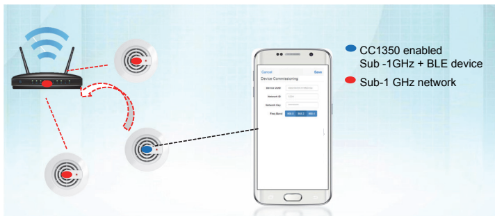
Figure 3: Bluetooth software: Fully connectable stack Sub-1 GHz software: TI 15.4-Stack or a legacy Sub-1 GHz solution.
