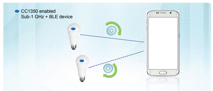
Figure 4: Bluetooth software: Fully connectable stack Sub-1 GHz software: TI 15.4-Stack or a legacy Sub-1 GHz solution.
