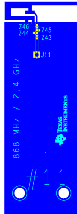
Figure 43. Board #11: 2.4 GHz PCB Antenna
