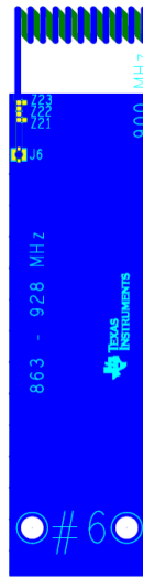
Figure 27. Board #6: Compact PCB Antenna
