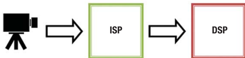
Figure 2. Typical embedded vision system, including camera, pre-processing FPGA and DSP.
