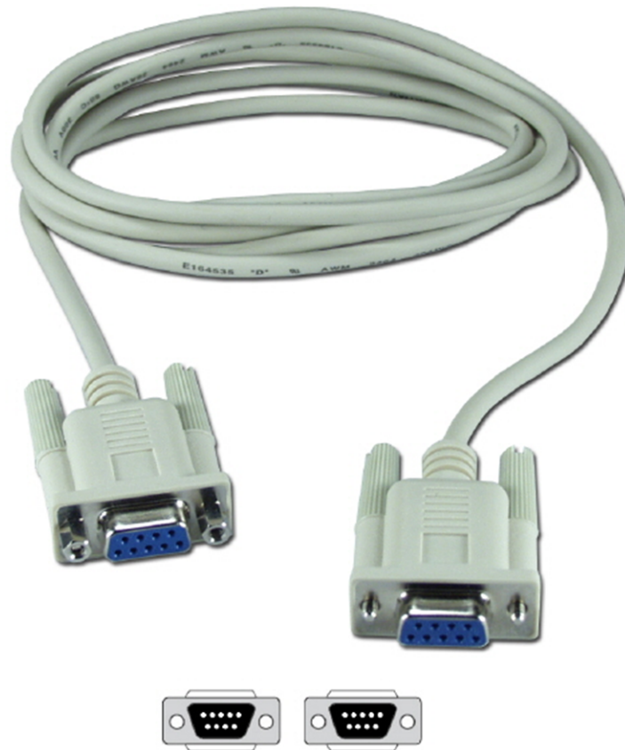
Figure 3-19. UART F-F Serial Cable
