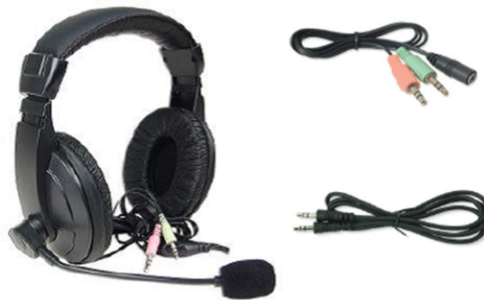
Figure 3-23. HP-Out, Mic-in, and Line-in Cables
