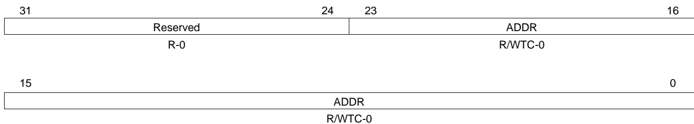
Figure 175. VBUSP DMA Bus Interface Status (VD_RD_BUSERR) Registers
