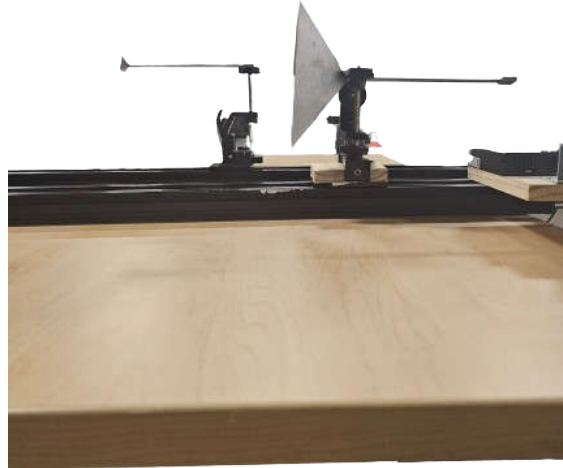
Figure 4-4. Image of Setup Used for Interference by Object Outside the Detection Zone Functional Test
