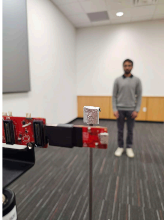
Figure 4-6. Image of Setup for Interference by Object Inside the Detection Zone
