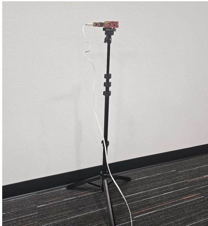
Figure 7-2. Picture of an IWR6843AOP on a Tripod That is Pointed at the Corner Reflector at the Required Distance per Test
