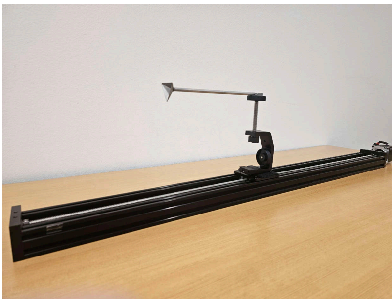
Figure 7-1. Picture of Linear Actuator setup With the Static Residual Movement's Specified Size Corner Reflector
