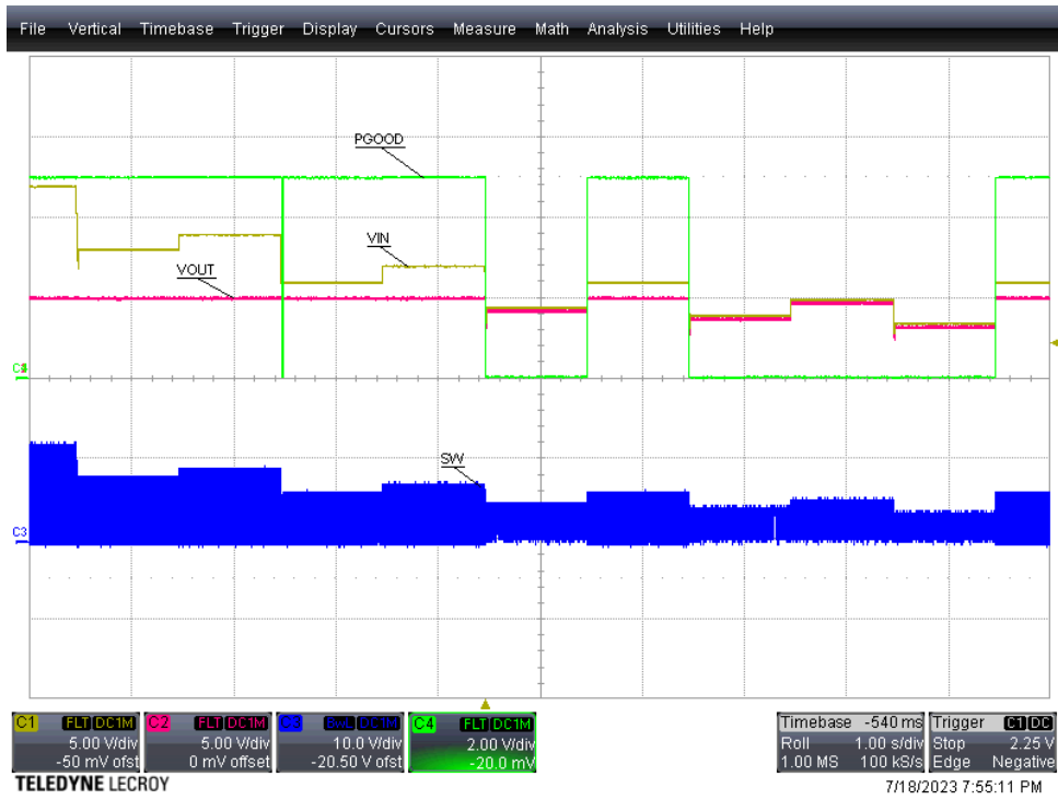
Figure 3-8. Waterfall Test, Iout = 300mA
