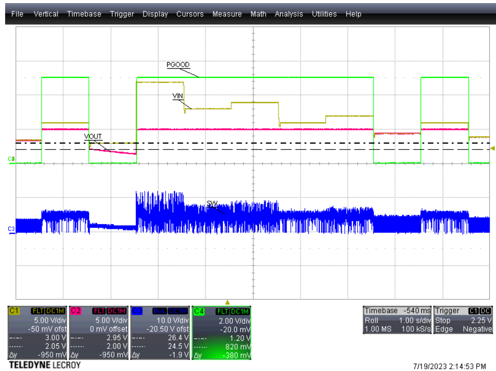
Figure 3-9. Waterfall Test, Iout = 0A
