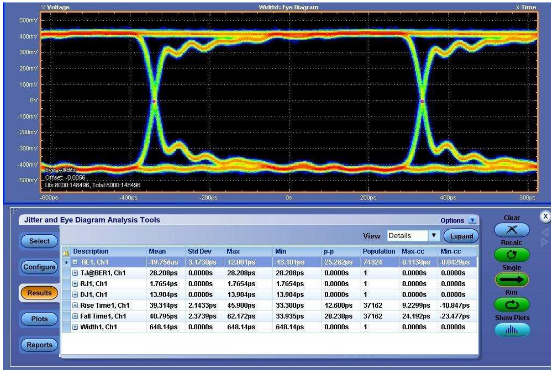
Figure 11. OUT0 (75 Ω) Alignment Jitter (AJ) and Rise / Fall Time at 1.485 Gbps AJ = 28.208 ps, Tr / Tf = 39.314 / 40.795 ps
