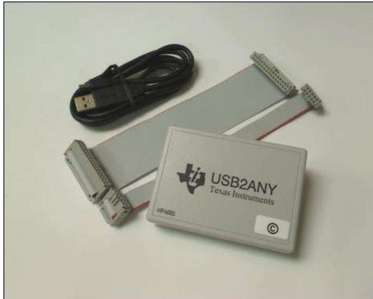
Figure 3. USB2ANY Interface for LMH1218EVM SPI and SMBus Control
