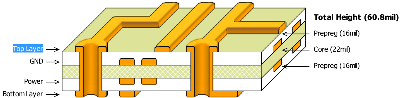
Figure 7. Board Layer Stack Up
