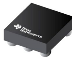
Figure 2. The HDC2010 humidity and temperature sensor is offered in a 1.5-mm × 1.5-mm WCSP footprint.
