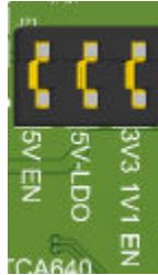
Figure 2-5. J21 Power Supply Control
