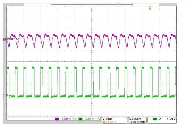
Figure 3-22. U2 Input Ripple – 3-A Load
