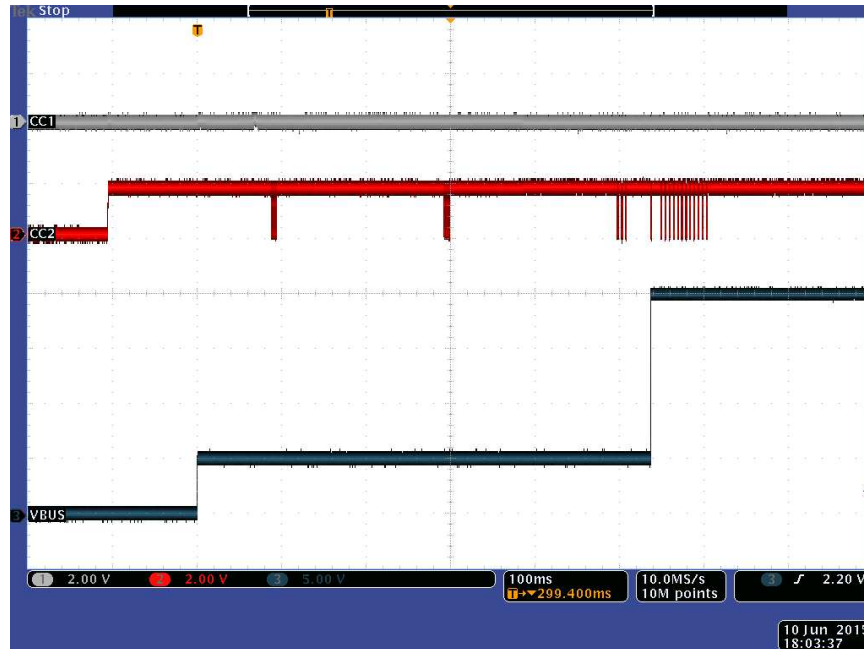
Figure 2. TPS65981 VBUS Voltage Transition
