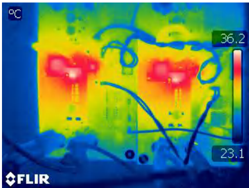
Figure 4-13. Thermal Condition in Boost Region ( V_{IN}=15V and 2A Load)
