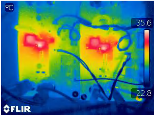
Figure 4-11. Thermal Condition in Boost Region ( V_{IN}=12V and 2A Load)
