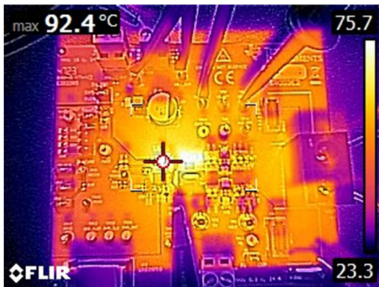
Figure 4-23. Thermal Characteristics, 800kHz FCCM, Internal LDO, 35A Load, no airflow, soak 10 minutes
