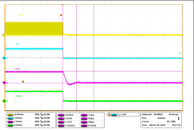
Figure 4-14. ENABLE Shutdown, 800kHz, 20A load
