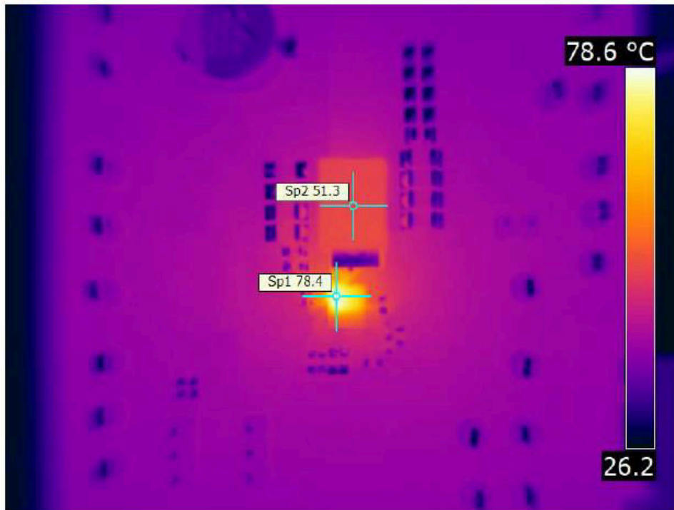
Figure 3-9. Thermal Image - 15-A load, T_{CASE} = 78.4^{\circ}\text{C} , T_{amb} = 25^{\circ}\text{C}
