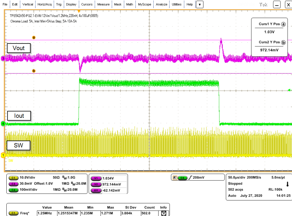
Figure 4-6. Transient response - 5-A to 10-A to 5-A load @ 5 \text{ A}/\mu\text{s} , \Delta V_{out} = 62.1 \text{ mV} , f_{sw} = 1200 kHz, FCCM
