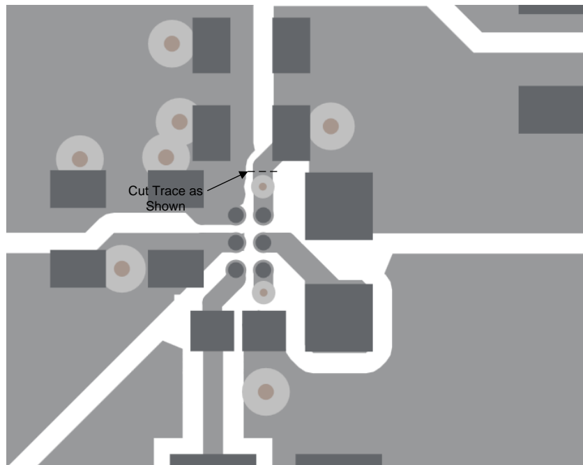
Figure 1. Loop Response Measurement Modification
