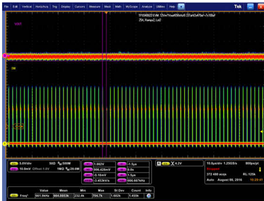
Figure 11-10. Output Ripple and SW Node of 1-V Output at 12 V IN , 25-A Output
