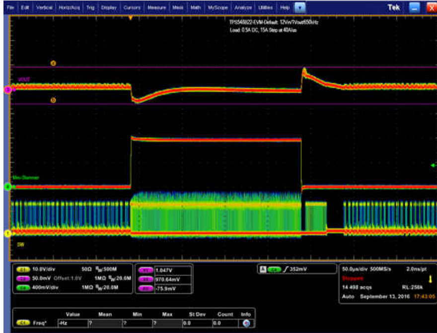
Figure 11-9. Transient Response of 1-V Output at 12 V IN , Transient is 0.5 A to 15.5 A, the Step is 15 A at 40 A/ \mu s
