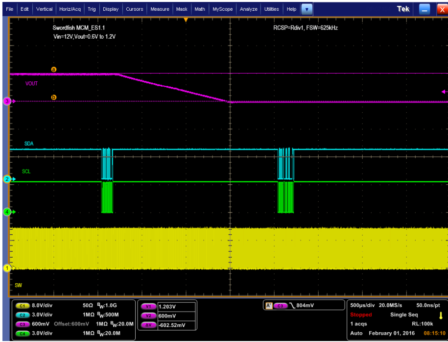
Figure 11-7. PMBus V_{OUT} Step-Down = 1.2 V to 0.6 V at 25 A
