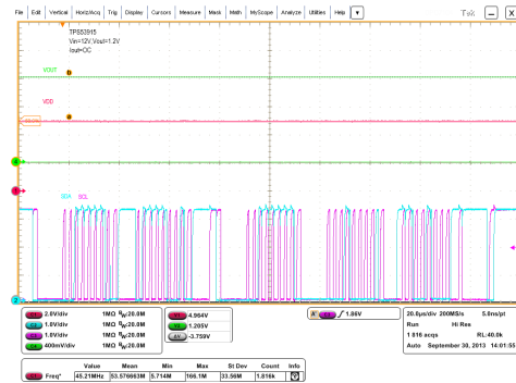
Figure 32. I 2 C READ (Address=31d, Cmd=0x79): ACK 0x10C8. I OC = 15 A
