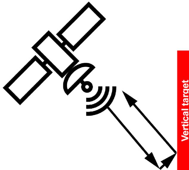
**Figure 2-2. Double Bounce of Radio Waves**
