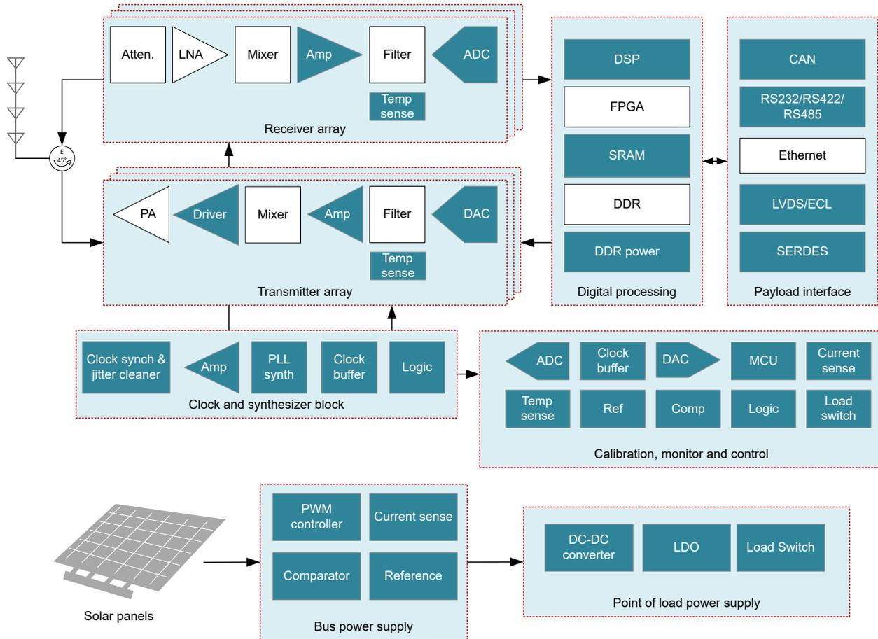
**Figure 2-3. Radar Imaging Payload Block Diagram**
