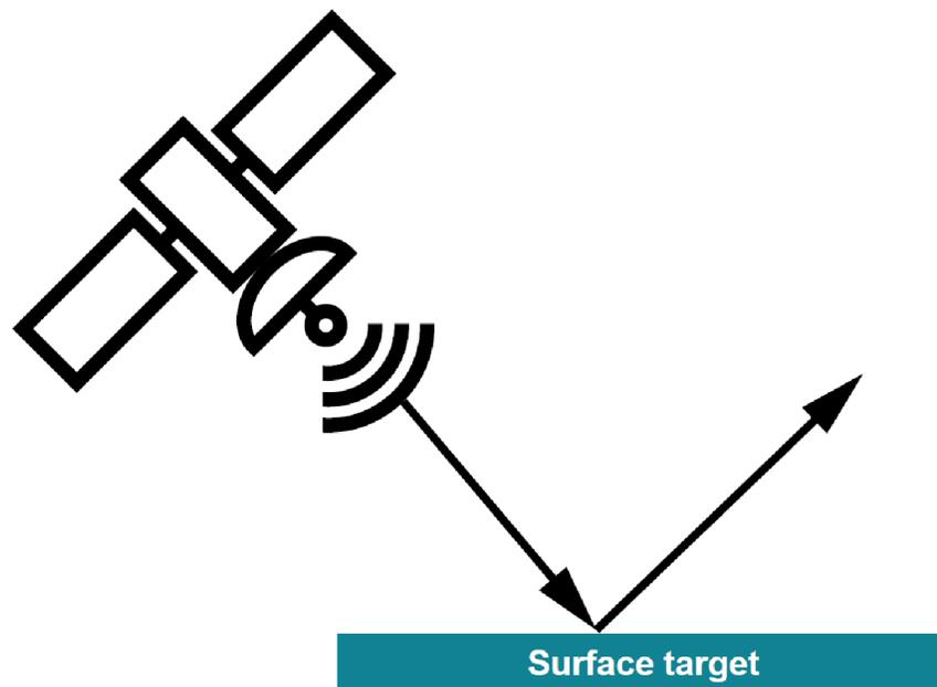
**Figure 2-1. Radio Waves Reflecting off a Smooth Surface Target**
