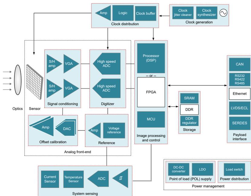
Figure 3-1. Optical imaging payload block diagram for passive sensing systems in satellites.
