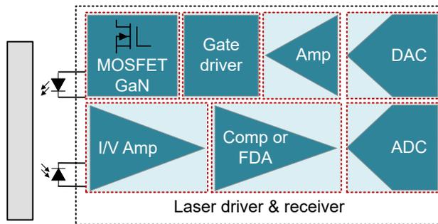
Figure 2-4. Laser Imaging Block Diagram
