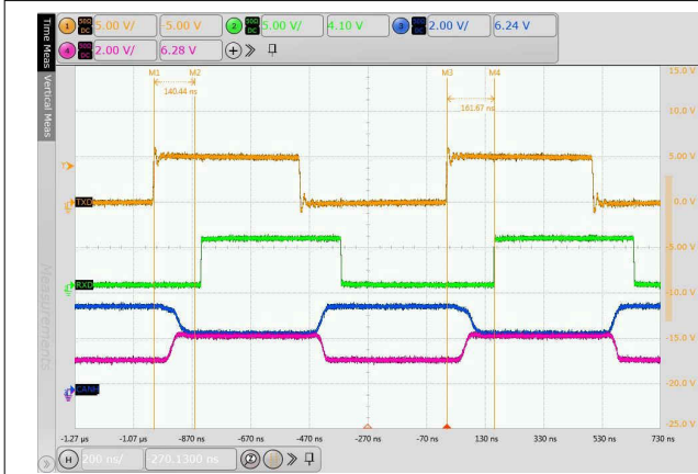
Figure 8-15. Typical TXD, RXD, CANH and CANL Waveforms at 2 Mbps
