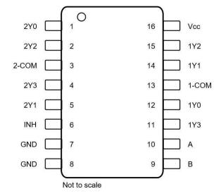
Figure 4-4. Pin Diagram SOT-23-THIN Package
