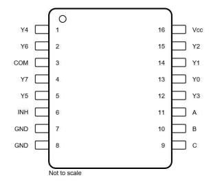
Figure 4-1. Pin Diagram TSSOP and SOIC Packages
