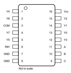
Figure 4-2. Pin Diagram SOT-23-THIN Package
