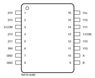
Figure 4-3. Pin Diagram TSSOP Package
