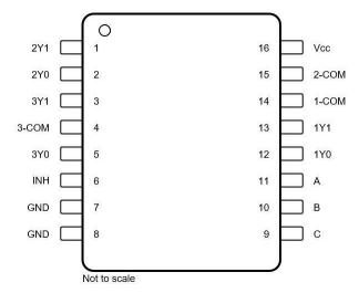
Figure 4-5. Pin Diagram TSSOP Package
