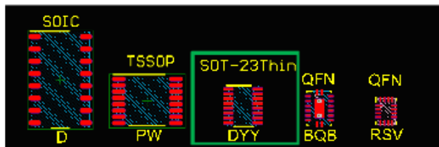
Figure 1. Packages Size Comparison - DYY Offers 57% Space Savings versus Legacy SOIC Package
