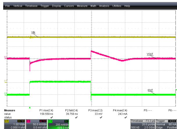
Figure 3-10. Current Probe Measurement with Shortened Cabling
