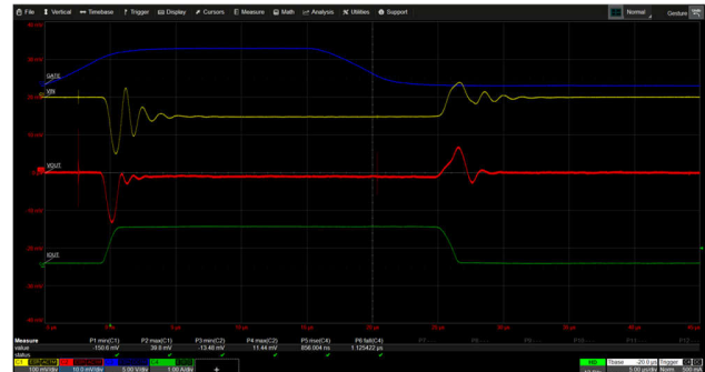
Figure 4-2. TPS7A96 Load Transient with Parasitic Limiting
