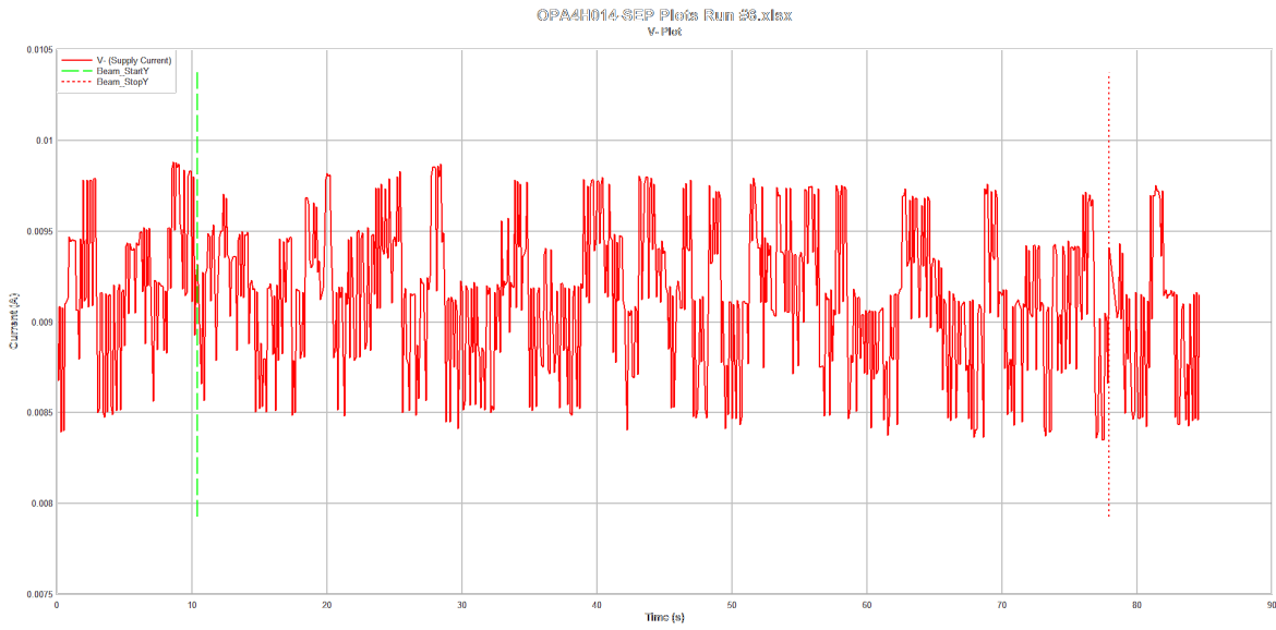
Figure 5-2. Current vs Time (I vs t) Data for V- Current During SEL Run 6
