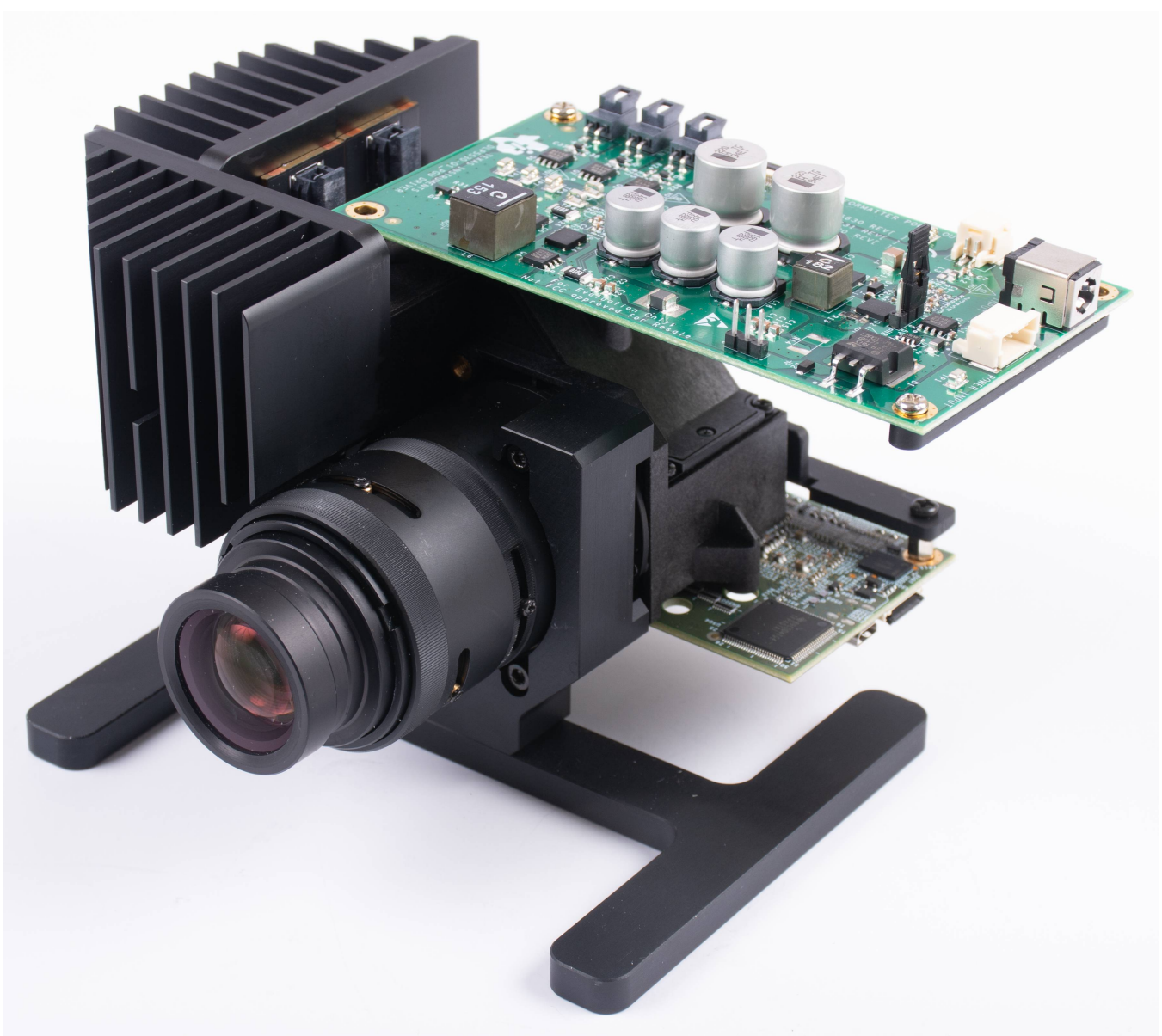
Figure 8. DLP5530PGUQ1EVM Optical Module
