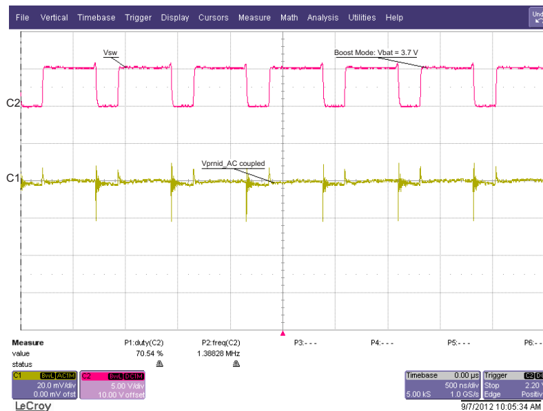
Figure 5. Boost Mode Ripple and Duty Cycle; V_{BAT} = 3.7 V
