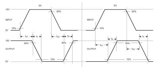
Figure 6-1. Switching Waveforms for (a) Inverting Driver and (b) Noninverting Driver
