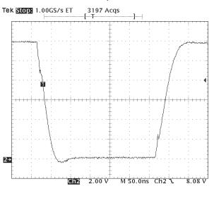
C<sub>L</sub> = 10 nF, C<sub>L</sub> = 10 nF, VDD = 12 V
