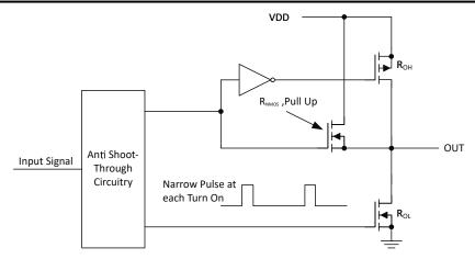
Figure 7-1. UCC27524 Gate Driver Output Structure
