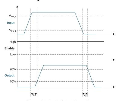
Figure 6-2. Input-Output Operation
