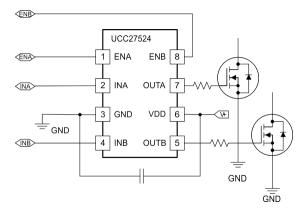
Figure 8-1. UCC27524 Typical Application Diagram
