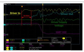
Vin = 210 V, Vout = 235 V, lout = 1.14 A, Fsw = 125 kHz, driver supply voltage = 15 V, gate resistor = 0  $\Omega$
