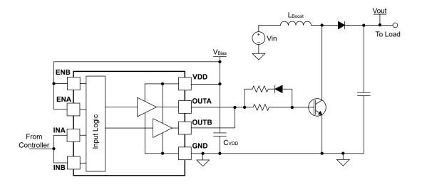
Figure 8-3. UCC27524 Used to Drive IGBT in the Boost Converter
