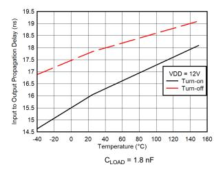
Figure 6-19. Input Propagation Delay vs Temperature
