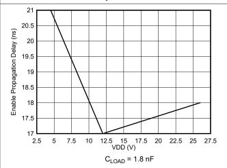
Figure 6-20. Enable to Output Rising Propagation Delay
