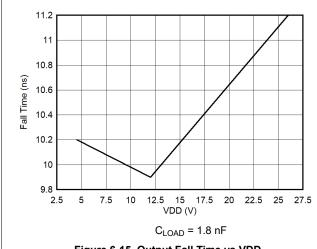
Figure 6-15. Output Fall Time vs VDD
