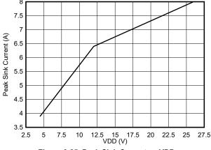
Figure 6-25. Peak Sink Current vs VDD
