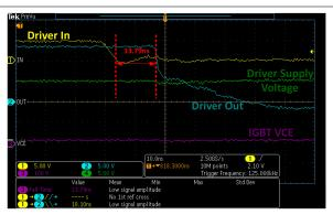
Vin = 210 V, Vout = 235 V, lout = 1.14 A, Fsw = 100 kHz, driver supply voltage = 15 V, gate resistor = 0  $\Omega$
