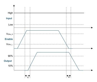
Figure 6-1. Enable Function
