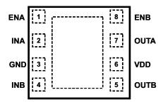
Figure 5-2. DSD Package 8-Pin WSON Top View
