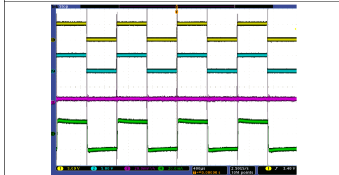
CH1: V_{(PWM3)} CH2: V_{(PWM4)} CH3: V_{(REF)} CH4: I_{(IOUT8)} Duty cycle = 50% V_{(SUPPLY)} , V_{(EN)} = 14\text{ V}
