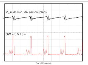
Figure 8-9. Input Voltage Ripple, I<sub>OUT</sub> = 700 mA
