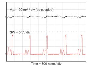
Figure 8-12. Output Voltage Ripple, I<sub>OUT</sub> = 700 mA
