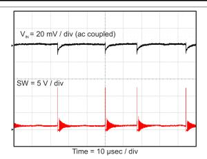
Figure 8-8. Input Voltage Ripple, I<sub>OUT</sub> = 10 mA
