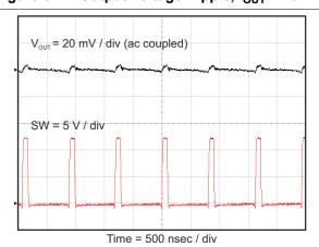
Figure 8-13. Output Voltage Ripple, I<sub>OUT</sub> = 8 A
