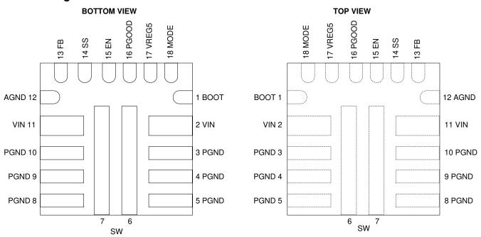
Figure 5-1. RNN Package 18-Pin VQFN
