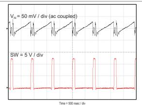
Figure 8-10. Input Voltage Ripple, I<sub>OUT</sub> = 8 A
