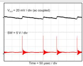
Figure 8-11. Output Voltage Ripple, I<sub>OUT</sub> = 10 mA
