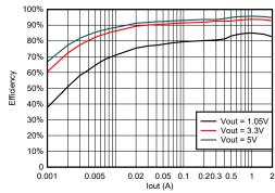
TPS562242 Efficiency at V<sub>IN</sub> = 12 V
