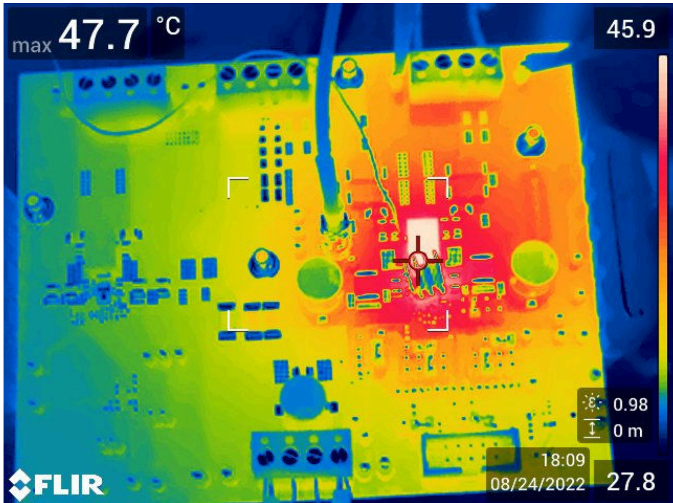
Figure 7-24. Thermal Image at 25°C Ambient
