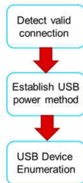
Figure 10-13. Flow of DFP-to-UFP Configuration
