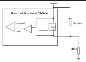
Figure 6-10. Open-Load Detection in Output Off
