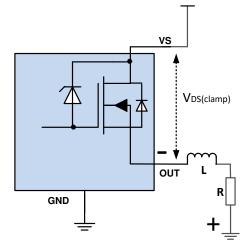
Figure 6-14. Drain-to-Source Clamping Structure
