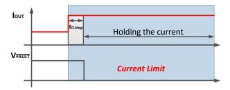
Figure 6-3. Holding Mode Example
