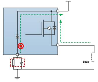
Figure 6-18. Reverse-Current External Protection, Method 2
