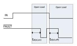
Figure 5-2. Open-Load Blanking-Time Characteristic
