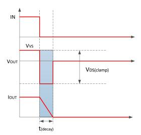
Figure 6-15. Inductive-Load Switching-Off Diagram
