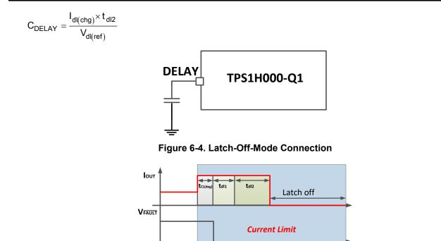
Figure 6-5. Latch-Off-Mode Example
