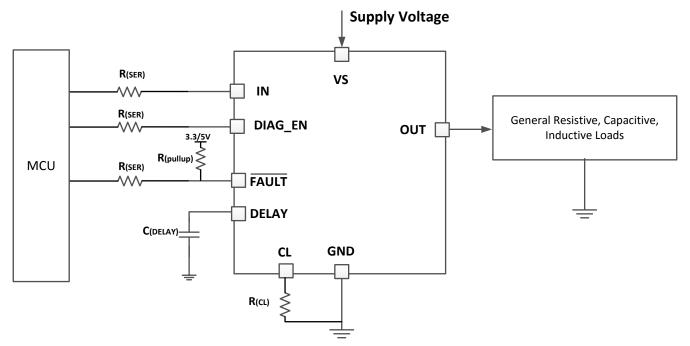
Figure 7-1. Typical Application Circuitry
