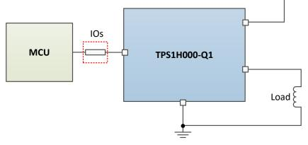
Figure 6-19. MCU I/O External Protection
