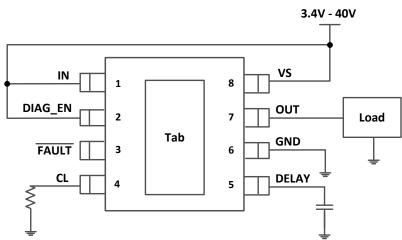
Figure 6-8. Standalone Operation in Latch-Off Mode
