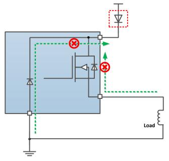
Figure 6-17. Reverse-Current External Protection, Method 1
