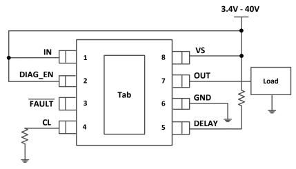
Figure 6-9. Standalone Operation in Auto-Retry Mode
