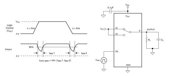
Figure 11. Break-Before-Make Delay Measurement Setup
