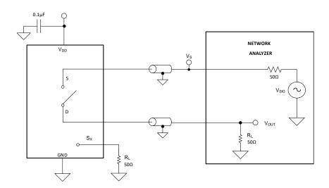
Figure 13. Off Isolation Measurement Setup
