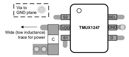
Figure 22. TMUX1247 Layout Example
