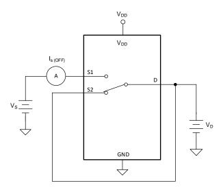
Figure 8. Off-Leakage Measurement Setup
