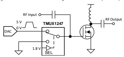
Figure 17. Input Control of Power Amplifier
