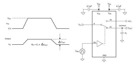
Figure 12. Charge-Injection Measurement Setup
