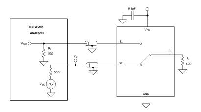
Figure 14. Crosstalk Measurement Setup
