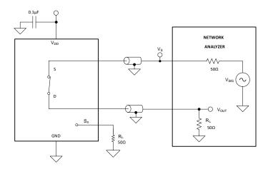
Figure 15. Bandwidth Measurement Setup
