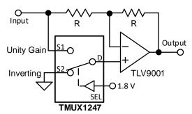
Figure 19. Switchable Op Amp Gain Setting
