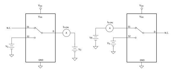
Figure 9. On-Leakage Measurement Setup
