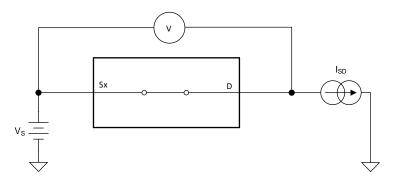
Figure 7. On-Resistance Measurement Setup
