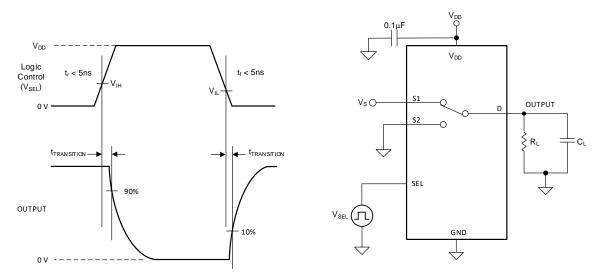
Figure 10. Transition-Time Measurement Setup
