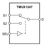
Figure 16. TMUX1247 Functional Block Diagram
