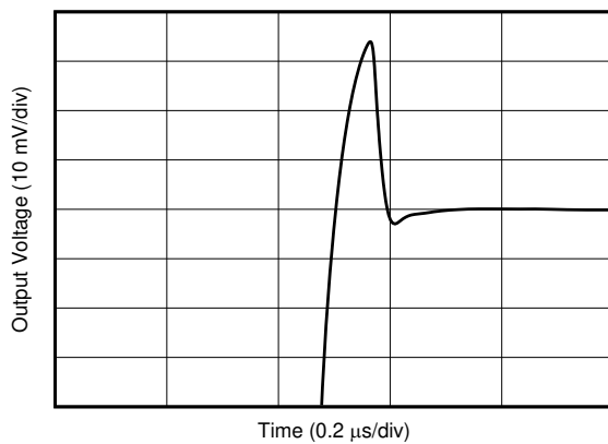
Figure 7-31. Small-Signal Step Response
