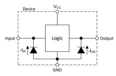
Figure 7-1. Electrical Placement of Clamping Diodes for Each Input and Output
