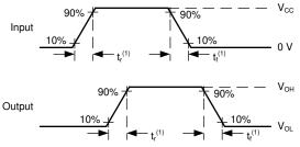
(1) The greater between  $t_{r}$  and  $t_{f}$  is the same as  $t_{t}. \label{eq:tf}$
