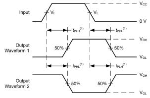
(1) The greater between  $t_{PLH}$  and  $t_{PHL}$  is the same as  $t_{pd}$ .
