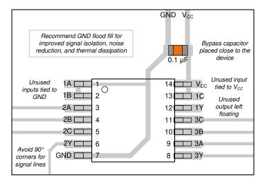
Figure 8-3. Example Layout for the SN74LVC11A-Q1
