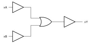
Simplified Logic Diagram (Positive Logic)
