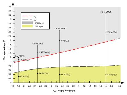
Figure 7-2. LVxT Input Voltage Levels
