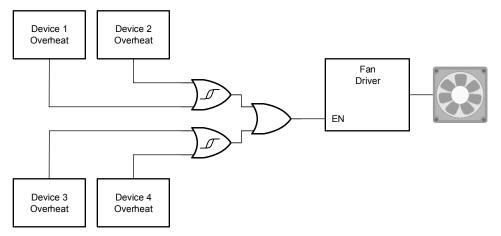
Figure 8-1. Typical Application Block Diagram
