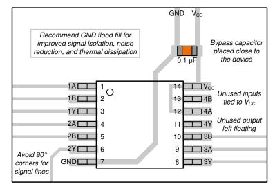
Figure 8-3. Example Layout for the SN74LV4T32-EP
