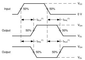
(1) The greater between t<sub>PLH</sub> and t<sub>PHL</sub> is the same as t<sub>pd</sub>. Figure 6-2. Voltage Waveforms Propagation Delays
