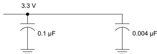
Figure 9-2. Recommended M-LVDS Bypass Capacitor Layout
