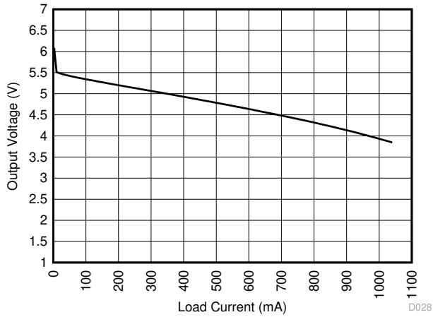
SN6505A + Würth 750316031 V_{CC} = 3.3\text{ V}
