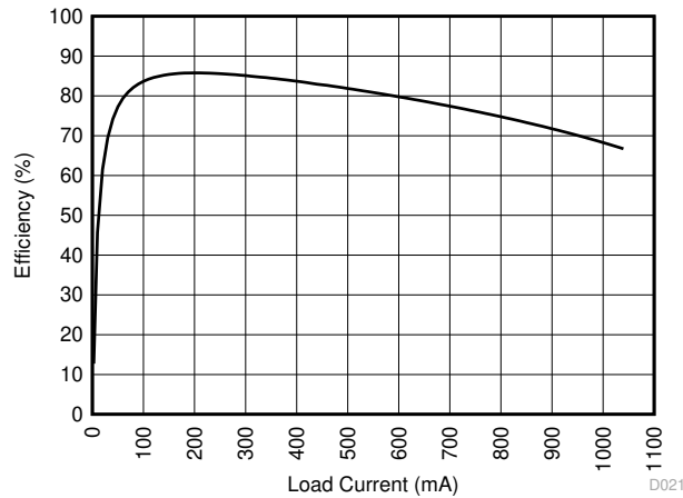
SN6505B + Würth 750316028 V_{CC} = 3.3\text{ V}
