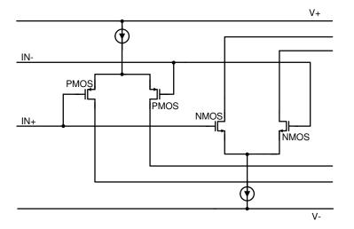
Figure 7-8. Rail-to-Rail Input Stage
