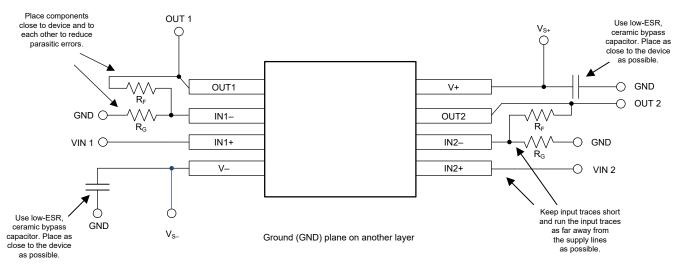
Figure 8-4. Operational Amplifier Board Layout for Noninverting Configuration
