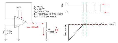
Figure 7-4. Thermal Protection
