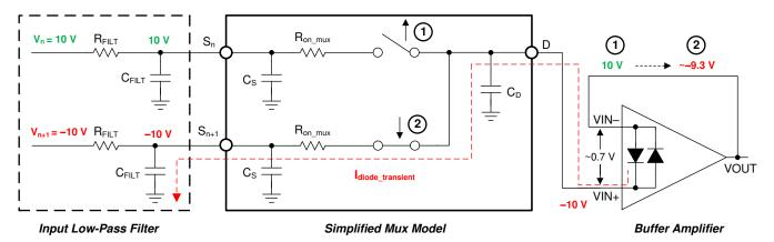
Figure 7-2. Back-to-Back Diodes Create Settling Issues
