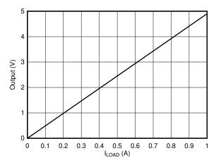
Figure 8-2. Low-Side, Current-Sense, Transfer Function
