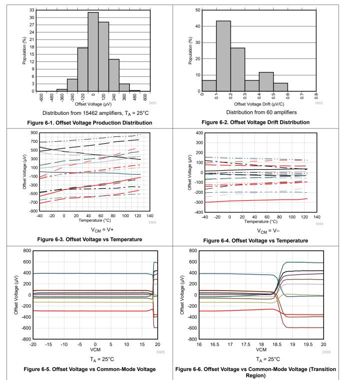
at  $T_A = 25^{\circ}C$ ,  $V_S = \pm 20$  V,  $V_{CM} = V_S / 2$ ,  $R_{LOAD} = 10$  k $\Omega$  connected to  $V_S / 2$ , and  $C_L = 10$  pF (unless otherwise noted)
