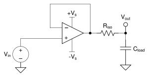
Figure 7-7. Extending Capacitive Load Drive With the OPA4H199-SEP
