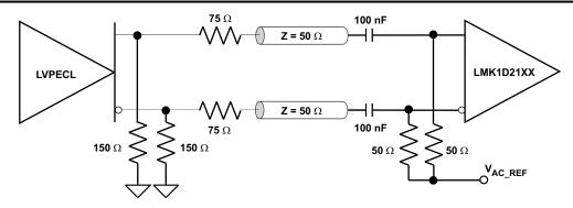
Figure 8-5. LVPECL Clock Driver Connected to LMK1D210x Input
