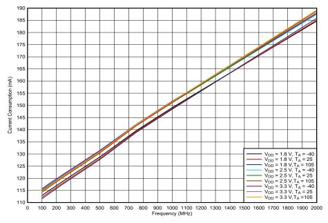
Figure 6-1. LMK1D2106 Current Consumption vs. Frequency, AMP\_SEL = 0
