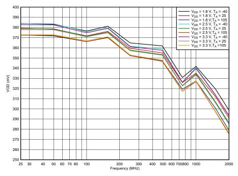
Figure 6-5. LMK1D210x VOD vs. Frequency, AMP\_SEL = 0
