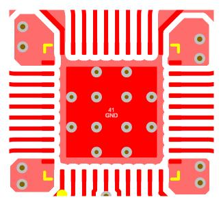
Figure 11-1. PCB layout example for LMK1D2106, Top Layer
