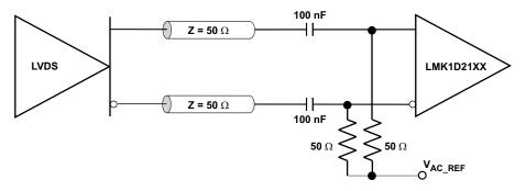
Figure 8-4. LVDS Clock Driver Connected to LMK1D210x Input (AC-Coupled)
