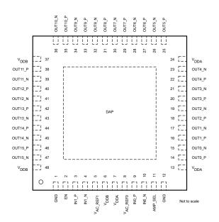
Figure 5-2. LMK1D2108: RGZ Package 48-Pin VQFN Top View
