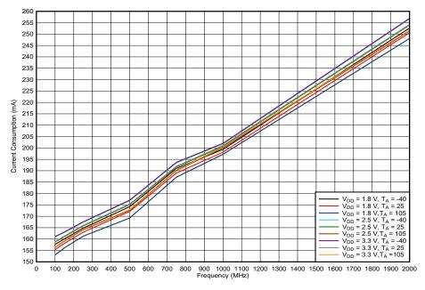
Figure 6-4. LMK1D2108 Current Consumption vs. Frequency, AMP\_SEL = 1
