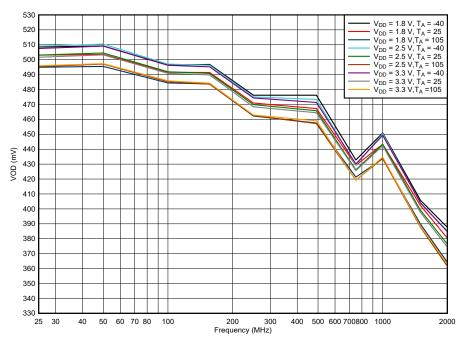
Figure 6-6. LMK1D210x VOD vs. Frequency, AMP\_SEL = 1
