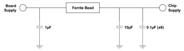
Figure 10-1. Power Supply Decoupling
