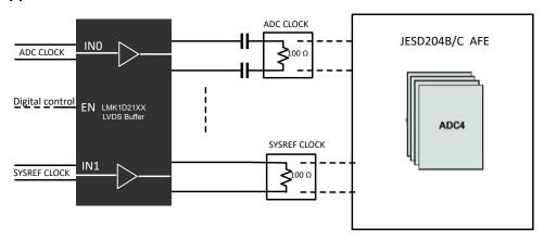
Figure 9-1. Fan-Out Buffer for ADC Device Clock and SYSREF Distribution
