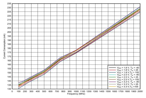
Figure 6-3. LMK1D2108 Current Consumption vs. Frequency, AMP\_SEL = 0
