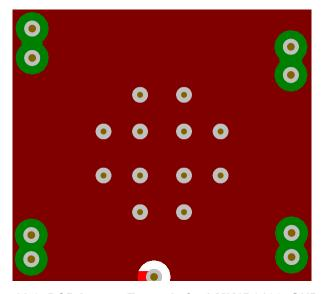
Figure 11-2. PCB Layout Example for LMK1D2106, GND layer
