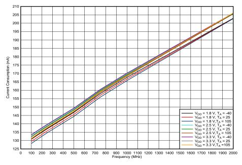
Figure 6-2. LMK1D2106 Current Consumption vs. Frequency, AMP\_SEL = 1
