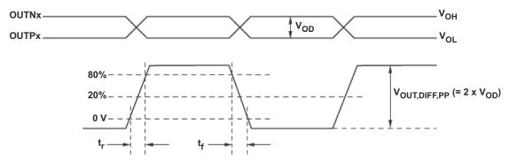
Figure 7-4. Output Voltage and Rise/Fall Time
